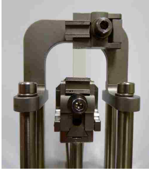
Figure 3.8: Specimen in Tension in DMA
